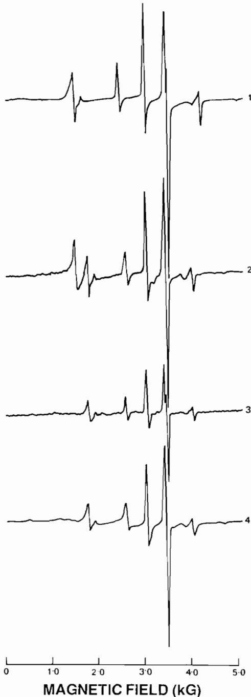
Fig. 7. First derivative ESR spectrum of a frozen dmf solution at 77 K of: (1) \text{Cr(III)(salhy)}_2 \cdot \text{NO}_3 \cdot \text{H}_2\text{O} ( 3.0 \times 10^{-3} mol \text{dm}^{-3} ); (2) \text{Cr(III)(salhy)}_2 \cdot \text{I} \cdot \text{H}_2\text{O} ; (3) \text{Cr(III)(salhy)}_2 \cdot \text{CN} \cdot \text{H}_2\text{O} ; (4) \text{Cr(III)(salhy)}_2 \cdot \text{SCN} \cdot \text{H}_2\text{O} . Microwave frequency 9.136 GHz.
